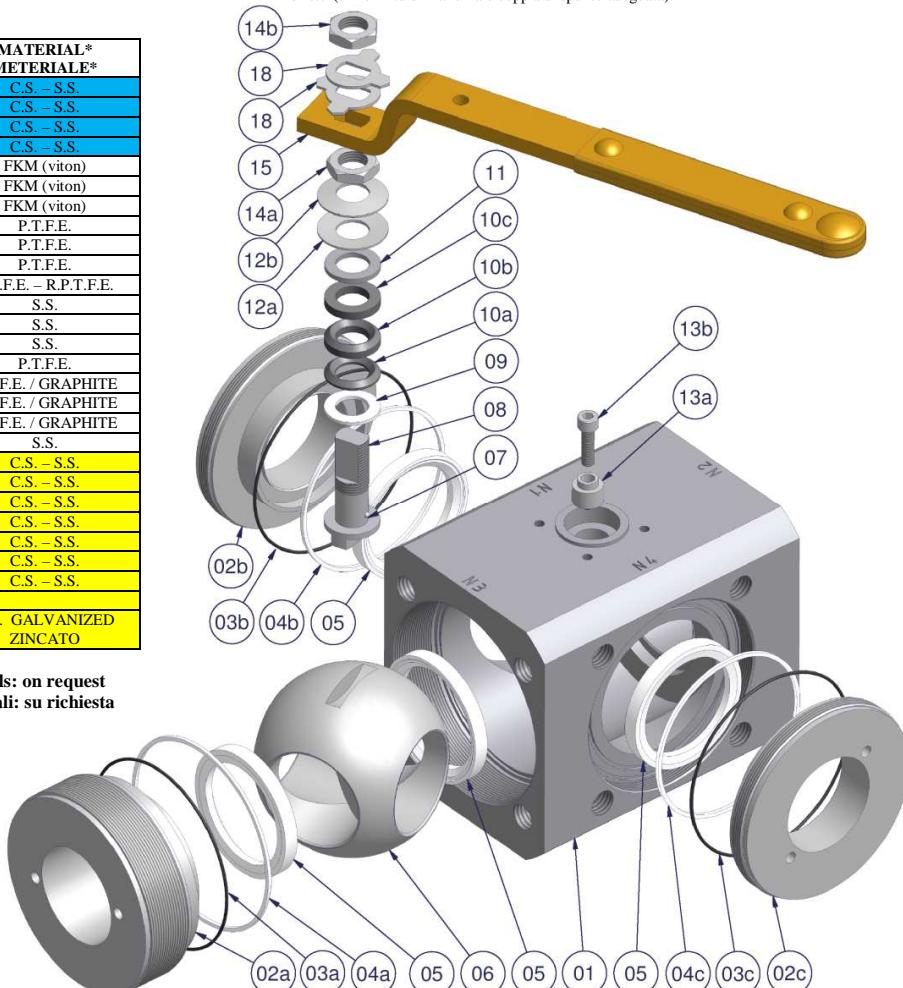
Considering working conditions, after a certain period of work and operations the ball valves may have problems of tightness due to seats & seals settlement. Small leakage from the stem can be solved adjusting stem bolts.
